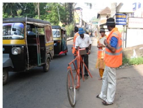
Plate 4 Roughness studies using MERLIN
