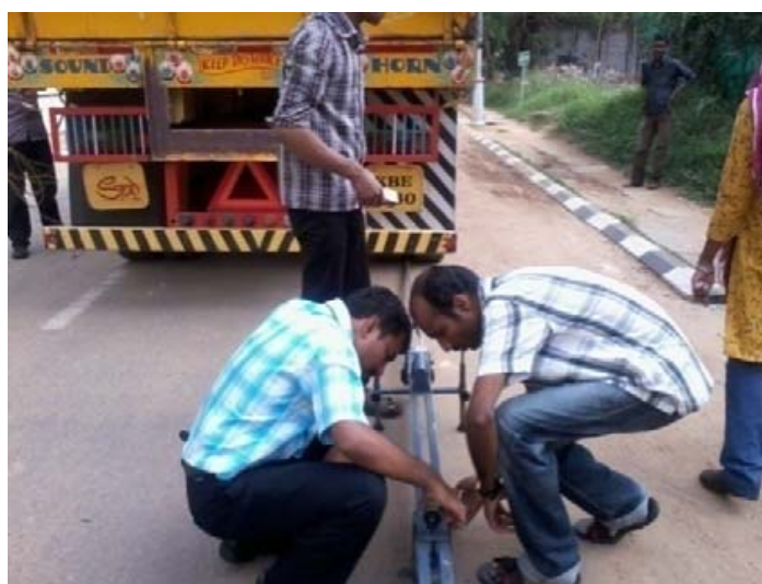
Plate 5 Setting of the Beam for BBD Survey
