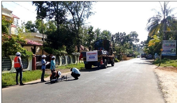
Figure 3 : Structural strength evaluation for existing pavement using Benkelman Beam Deflection
