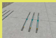
Dowelbar For inter connection
