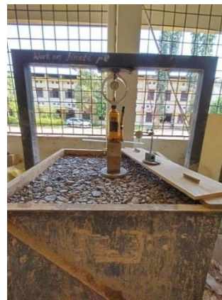
Plate Load Test Setup
