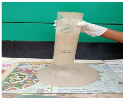
Flowability Measurement from the spread diameter
