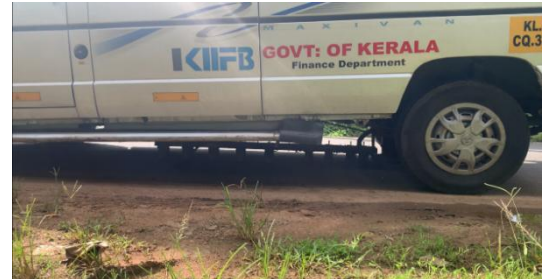
Pavement Structural Evaluation using FWD
