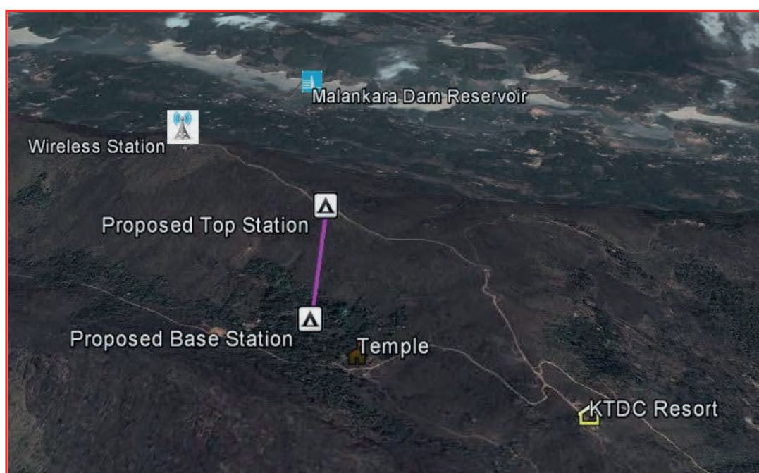
Figure 16: Map Showing the Final Alignment Chosen for Ropeway System
